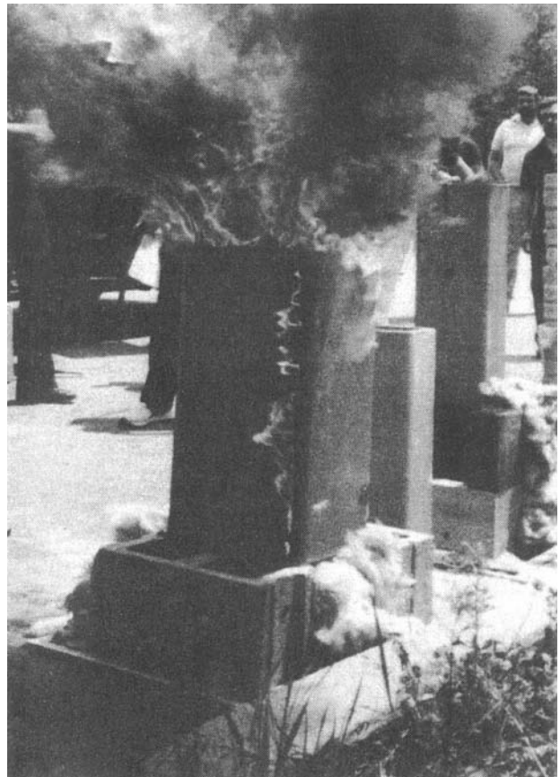
Figure 3-9. In this photograph of a demonstration chimney fire, a clay flue liner, its interior coated with tar, has been ignited to simulate a chimney fire. Notice the severe crack at the near corner and the flame escaping the confines of the liner.
